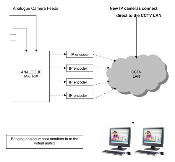
6.11 The schematic above illustrates how the concept of connecting the analogue matrix to the virtual matrix and spot monitors. The next step could be to connect the virtual matrix to the 'wonderwall' (this would probably be the point
